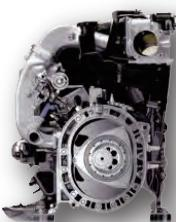
MAZDA Hydrogen rotary engine
